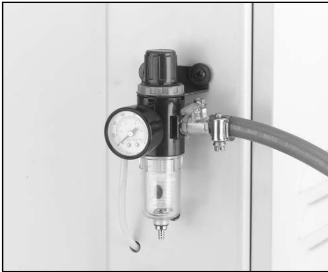
Figure 10. Secure air hose with a hose clamp.
